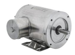
IronHorse MTS premium efficiency AC induction motor, washdown and inverter rated, 3/4hp, 3-phase, 208-230/460 VAC, 1800rpm, TENV, NEMA 56C frame, 304 stainless steel, C-face/rigid base mount.
