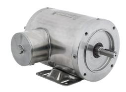
IronHorse MTS premium efficiency AC induction motor, washdown and inverter rated, 3/4hp, 3-phase, 208-230/460 VAC, 1800rpm, TENV, 56C frame, 304 stainless steel, C-face/rigid base mount.
