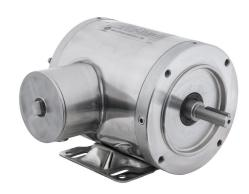
IronHorse MTS premium efficiency AC induction motor, washdown and inverter rated, 1/2hp, 3-phase, 208-230/460 VAC, 3600rpm, TENV, NEMA 56C frame, 304 stainless steel, C-face/rigid base mount.
