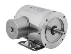
IronHorse MTS premium efficiency AC induction motor, washdown and inverter rated, 1/2hp, 3-phase, 208-230/460 VAC, 1800rpm, TENV, NEMA 56C frame, 304 stainless steel, C-face/rigid base mount.
