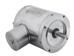
IronHorse MTS premium efficiency AC induction motor, washdown and inverter rated, 1/2hp, 3-phase, 208-230/460 VAC, 1800rpm, TENV, NEMA 56C frame, 304 stainless steel, C-face mount.
