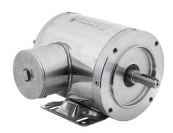
IronHorse MTS premium efficiency AC induction motor, washdown and inverter rated, 1/3hp, 3-phase, 208-230/460 VAC, 3600rpm, TENV, NEMA 56C frame, 304 stainless steel, C-face/rigid base mount.
