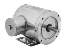
IronHorse MTS premium efficiency AC induction motor, washdown and inverter rated, 1/3hp, 3-phase, 208-230/460 VAC, 1800rpm, TENV, NEMA 56C frame, 304 stainless steel, C-face/rigid base mount.
