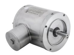
IronHorse MTS premium efficiency AC induction motor, washdown and inverter rated, 1/3hp, 3-phase, 208-230/460 VAC, 1800rpm, TENV, NEMA 56C frame, 304 stainless steel, C-face mount.
