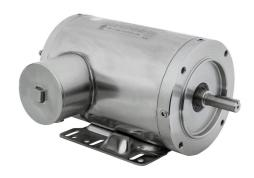
IronHorse MTS premium efficiency AC induction motor, washdown and inverter rated, 1-1/2hp, 3-phase, 208-230/460 VAC, 3600rpm, TENV, 56C frame, 304 stainless steel, C-face/rigid base mount.
