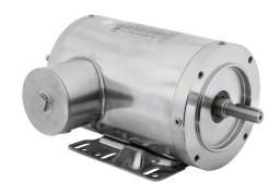
IronHorse MTS premium efficiency AC induction motor, washdown and inverter rated, 1-1/2hp, 3-phase, 208-230/460 VAC, 1800rpm, TENV, 56C frame, 304 stainless steel, C-face/rigid base mount.
