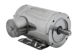
IronHorse MTS premium efficiency AC induction motor, washdown and inverter rated, 1-1/2hp, 3-phase, 208-230/460 VAC, 1800rpm, TENV, NEMA 145TC frame, 304 stainless steel, C-face/rigid base mount.
