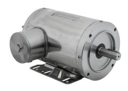
IronHorse MTS premium efficiency AC induction motor, washdown and inverter rated, 1-1/2hp, 3-phase, 208-230/460 VAC, 1800rpm, TENV, 145TC frame, 304 stainless steel, C-face/rigid base mount.
