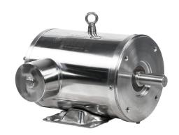
IronHorse MTS premium efficiency AC induction motor, washdown and inverter rated, 3hp, 3-phase, 208-230/460 VAC, 1800rpm, TENV, NEMA 182TC frame, 304 stainless steel, C-face/rigid base mount.
