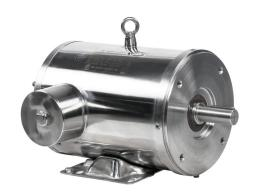
IronHorse MTS premium efficiency AC induction motor, washdown and inverter rated, 3hp, 3-phase, 208-230/460 VAC, 1800rpm, TENV, 182TC frame, 304 stainless steel, C-face/rigid base mount.
