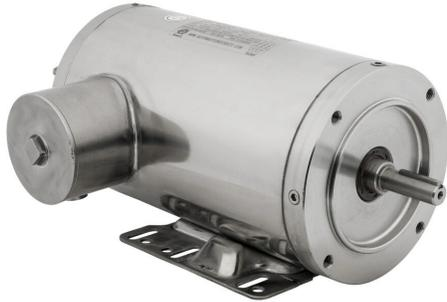
IronHorse MTS premium efficiency AC induction motor, washdown and inverter rated, 2hp, 3-phase, 208-230/460 VAC, 3600rpm, TENV, NEMA 56C frame, 304 stainless steel, C-face/rigid base mount.
