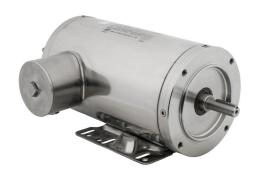
IronHorse MTS premium efficiency AC induction motor, washdown and inverter rated, 2hp, 3-phase, 208-230/460 VAC, 3600rpm, TENV, 56C frame, 304 stainless steel, C-face/rigid base mount.
