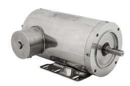
IronHorse MTS premium efficiency AC induction motor, washdown and inverter rated, 2hp, 3-phase, 208-230/460 VAC, 1800rpm, TENV, NEMA 56C frame, 304 stainless steel, C-face/rigid base mount.
