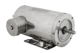
IronHorse MTS premium efficiency AC induction motor, washdown and inverter rated, 2hp, 3-phase, 208-230/460 VAC, 1800rpm, TENV, 56C frame, 304 stainless steel, C-face/rigid base mount.
