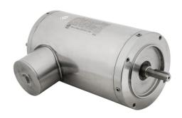
IronHorse MTS premium efficiency AC induction motor, washdown and inverter rated, 2hp, 3-phase, 208-230/460 VAC, 1800rpm, TENV, NEMA 56C frame, 304 stainless steel, C-face mount.
