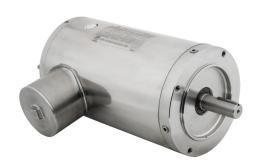
IronHorse MTS premium efficiency AC induction motor, washdown and inverter rated, 2hp, 3-phase, 208-230/460 VAC, 1800rpm, TENV, NEMA 145TC frame, 304 stainless steel, C-face mount.
