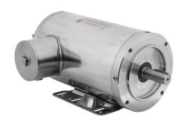
IronHorse MTS premium efficiency AC induction motor, washdown and inverter rated, 2hp, 3-phase, 208-230/460 VAC, 1800rpm, TENV, NEMA 145TC frame, 304 stainless steel, C-face/rigid base mount.
