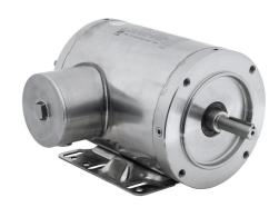
IronHorse MTS premium efficiency AC induction motor, washdown and inverter rated, 1hp, 3-phase, 208-230/460 VAC, 3600rpm, TENV, NEMA 56C frame, 304 stainless steel, C-face/rigid base mount.
