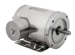
IronHorse MTS premium efficiency AC induction motor, washdown and inverter rated, 1hp, 3-phase, 208-230/460 VAC, 1800rpm, TENV, NEMA 56C frame, 304 stainless steel, C-face/rigid base mount.
