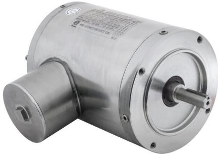
IronHorse MTS premium efficiency AC induction motor, washdown and inverter rated, 1hp, 3-phase, 208-230/460 VAC, 1800rpm, TENV, NEMA 56C frame, 304 stainless steel, C-face mount.
