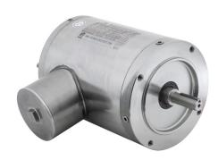
IronHorse MTS premium efficiency AC induction motor, washdown and inverter rated, 1hp, 3-phase, 208-230/460 VAC, 1800rpm, TENV, NEMA 56C frame, 304 stainless steel, C-face mount.
