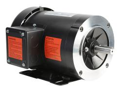
IronHorse MTR premium efficiency AC induction motor, general purpose and inverter rated, 1-1/2hp, 3-phase, 208-230/460 VAC, 3600rpm, TEFC, NEMA 56C/HC frame, rolled steel, C-face/ removable rigid base mount.
