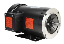
IronHorse MTR premium efficiency AC induction motor, general purpose and inverter rated, 1-1/2hp, 3-phase, 208-230/460 VAC, 1800rpm, TEFC, NEMA 56C/HC frame, rolled steel, C-face/removable rigid base mount.
