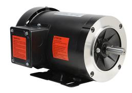
IronHorse MTR premium efficiency AC induction motor, general purpose and inverter rated, 3hp, 3-phase, 208-230/460 VAC, 3600rpm, TEFC, 56C/HC frame, rolled steel, C-face/removable rigid base mount.
