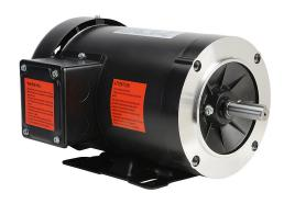
IronHorse MTR premium efficiency AC induction motor, general purpose and inverter rated, 3hp, 3-phase, 208-230/460 VAC, 3600rpm, TEFC, NEMA 56C/HC frame, rolled steel, C-face/removable rigid base mount.
