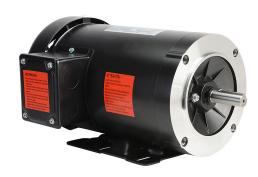
IronHorse MTR premium efficiency AC induction motor, general purpose and inverter rated, 2hp, 3-phase, 208-230/460 VAC, 1800rpm, TEFC, NEMA 56C/HC frame, rolled steel, C-face/removable rigid base mount.
