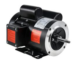
IronHorse MTR standard efficiency AC induction motor, centrifugal jet pump, 1-1/2hp, 1-phase, 115/230 VAC, 3600rpm, TEFC, NEMA 56J frame, rolled steel, C-face/removable rigid base mount.
