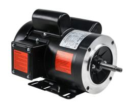
IronHorse MTR standard efficiency AC induction motor, centrifugal jet pump, 2hp, 1-phase, 115/230 VAC, 3600rpm, TEFC, NEMA 56J frame, rolled steel, C-face/removable rigid base mount.
