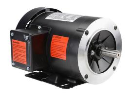
IronHorse MTR standard efficiency AC induction motor, general purpose and inverter rated, 3/4hp, 3-phase, 230/460 VAC, 3600rpm, TEFC, NEMA 56C frame, rolled steel, C-face/removable rigid base mount.
