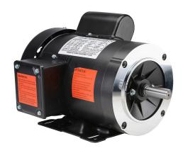
IronHorse MTR standard efficiency AC induction motor, general purpose, 3/4hp, 1-phase, 115/230 VAC, 1800rpm, TEFC, NEMA 56C frame, rolled steel, C-face/removable rigid base mount.
