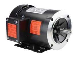
IronHorse MTR standard efficiency AC induction motor, general purpose and inverter rated, 1/2hp, 3-phase, 230/460 VAC, 3600rpm, TEFC, NEMA 56C frame, rolled steel, C-face/removable rigid base mount.
