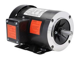
IronHorse MTR standard efficiency AC induction motor, general purpose and inverter rated, 1/2hp, 3-phase, 230/460 VAC, 1800rpm, TEFC, NEMA 56C frame, rolled steel, C-face/removable rigid base mount.
