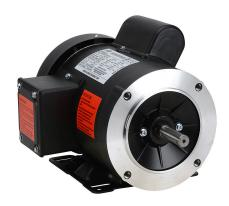
IronHorse MTR standard efficiency AC induction motor, general purpose, 1/2hp, 1-phase, 115/230 VAC, 3600rpm, TEFC, 56C frame, rolled steel, C-face/removable rigid base mount.
