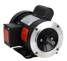
IronHorse MTR standard efficiency AC induction motor, general purpose, 1/2hp, 1-phase, 115/230 VAC, 3600rpm, TEFC, NEMA 56C frame, rolled steel, C-face/removable rigid base mount.
