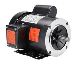
IronHorse MTR standard efficiency AC induction motor, general purpose, 1/2hp, 1-phase, 115/230 VAC, 1800rpm, TEFC, 56C frame, rolled steel, C-face/removable rigid base mount.
