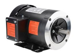
IronHorse MTR standard efficiency AC induction motor, general purpose and inverter rated, 1/3hp, 3-phase, 230/460 VAC, 1800rpm, TEFC, 56C frame, rolled steel, C-face/removable rigid base mount.
