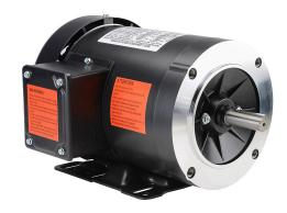
IronHorse MTR standard efficiency AC induction motor, general purpose and inverter rated, 1/3hp, 3-phase, 230/460 VAC, 1800rpm, TEFC, NEMA 56C frame, rolled steel, C-face/removable rigid base mount.
