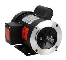
IronHorse MTR standard efficiency AC induction motor, general purpose, 1/3hp, 1-phase, 115/230 VAC, 3600rpm, TEFC, NEMA 56C frame, rolled steel, C-face/removable rigid base mount.
