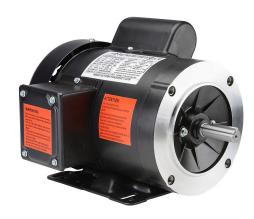
IronHorse MTR standard efficiency AC induction motor, general purpose, 1/3hp, 1-phase, 115/230 VAC, 1800rpm, TEFC, NEMA 56C frame, rolled steel, C-face/removable rigid base mount.
