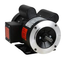
IronHorse MTR standard efficiency AC induction motor, general purpose, 1-1/2hp, 1-phase, 115/230 VAC, 3600rpm, TEFC, NEMA 56C frame, rolled steel, C-face/removable rigid base mount.
