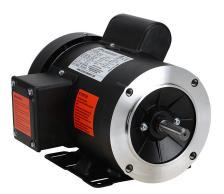
IronHorse MTR standard efficiency AC induction motor, general purpose, 1hp, 1-phase, 115/230 VAC, 3600rpm, TEFC, NEMA 56C frame, rolled steel, C-face/removable rigid base mount.
