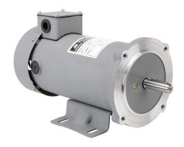
IronHorse MTPM DC permanent magnet motor, SCR-PWM rated, 3/4hp, 180 VDC, 1800rpm, TEFC, NEMA 56C frame, rolled steel, C-face/removable rigid base mount. Replacement brushes included.
