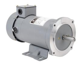
IronHorse MTPM DC permanent magnet motor, SCR-PWM rated, 3/4hp, 90 VDC, 1800rpm, TEFC, NEMA 56C frame, rolled steel, C-face/removable rigid base mount. Replacement brushes included.
