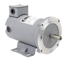
IronHorse MTPM DC permanent magnet motor, SCR-PWM rated, 1/2hp, 180 VDC, 1800rpm, TENV, 56C frame, rolled steel, C-face/removable rigid base mount. Replacement brushes included.
