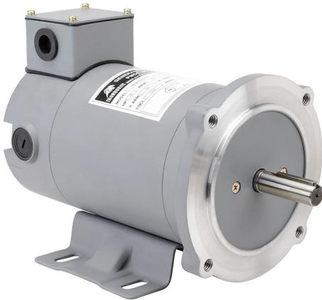
IronHorse MTPM DC permanent magnet motor, SCR-PWM rated, 1/2hp, 180 VDC, 1800rpm, TENV, NEMA 56C frame, rolled steel, C-face/removable rigid base mount. Replacement brushes included.
