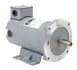
IronHorse MTPM DC permanent magnet motor, SCR-PWM rated, 1/2hp, 180 VDC, 1800rpm, TENV, NEMA 56C frame, rolled steel, C-face/removable rigid base mount. Replacement brushes included.
