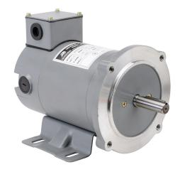
IronHorse MTPM DC permanent magnet motor, SCR-PWM rated, 1/3hp, 180 VDC, 1800rpm, TENV, NEMA 56C frame, rolled steel, C-face/removable rigid base mount. Replacement brushes included.
