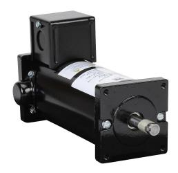
IronHorse MTPM DC permanent magnet motor, SCR-PWM rated, 1/4hp, 12/24 VDC, 1854/4375rpm, TENV, small frame, rolled steel, flange mount.
