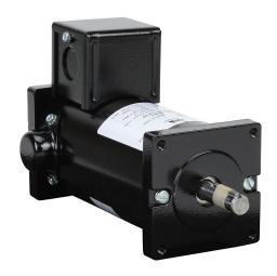
IronHorse MTPM DC permanent magnet motor, SCR-PWM rated, 1/4hp, 12/24 VDC, 1732/3996rpm, TENV, small frame, rolled steel, flange mount.
