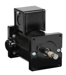
IronHorse MTPM DC permanent magnet motor, SCR-PWM rated, 1/6hp, 12/24 VDC, 1841/4290rpm, TENV, small frame, rolled steel, flange mount.
