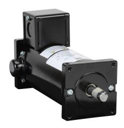
IronHorse MTPM DC permanent magnet motor, SCR-PWM rated, 1/7hp, 180 VDC, 1828rpm, TENV, small frame, rolled steel, flange mount.
