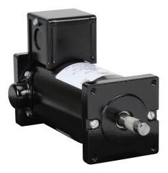
IronHorse MTPM DC permanent magnet motor, SCR-PWM rated, 1/8hp, 180 VDC, 1865rpm, TENV, small frame, rolled steel, flange mount.
