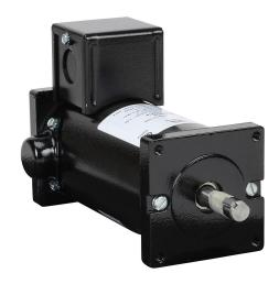
IronHorse MTPM DC permanent magnet motor, SCR-PWM rated, 1/8hp, 180 VDC, 1865rpm, TENV, small frame, rolled steel, flange mount.
