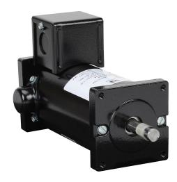
IronHorse MTPM DC permanent magnet motor, SCR-PWM rated, 1/8hp, 90 VDC, 1917rpm, TENV, small frame, rolled steel, flange mount.
