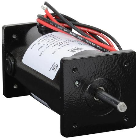
IronHorse MTPM DC permanent magnet motor, SCR-PWM rated, 1/8hp, 12/24 VDC, 1825/4224rpm, TENV, small frame, rolled steel, flange mount.
