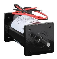
IronHorse MTPM DC permanent magnet motor, SCR-PWM rated, 1/10hp, 12/24 VDC, 1746/4252rpm, TENV, small frame, rolled steel, flange mount.
