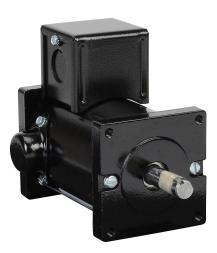
IronHorse MTPM DC permanent magnet motor, SCR-PWM rated, 1/19hp, 90 VDC, 1917rpm, TENV, small frame, rolled steel, flange mount.
