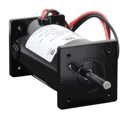
IronHorse MTPM DC permanent magnet motor, SCR-PWM rated, 1/26hp, 90 VDC, 1749rpm, TENV, small frame, rolled steel, flange mount.
